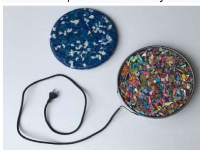
A machine was built with some pizza baking trays to produce little bench seats.
